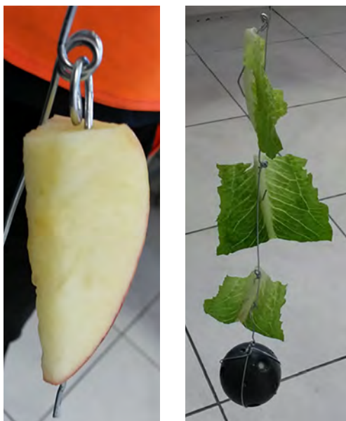
Figure 2. Apple slices and Romaine lettuce pieces on wire hooks used to extend the time in the UV Turbulator.
