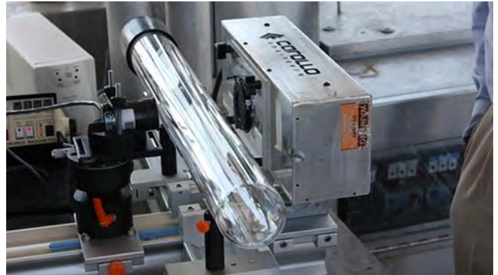
Figure 5. Custom optic bench for direct measurement of sleeve transmittance and fouling
