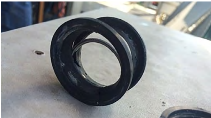
Figure 2. Broken wiper seals with exposed springs
