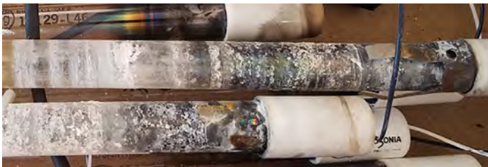
Figure 1. Lamp end darkening and corrosion
