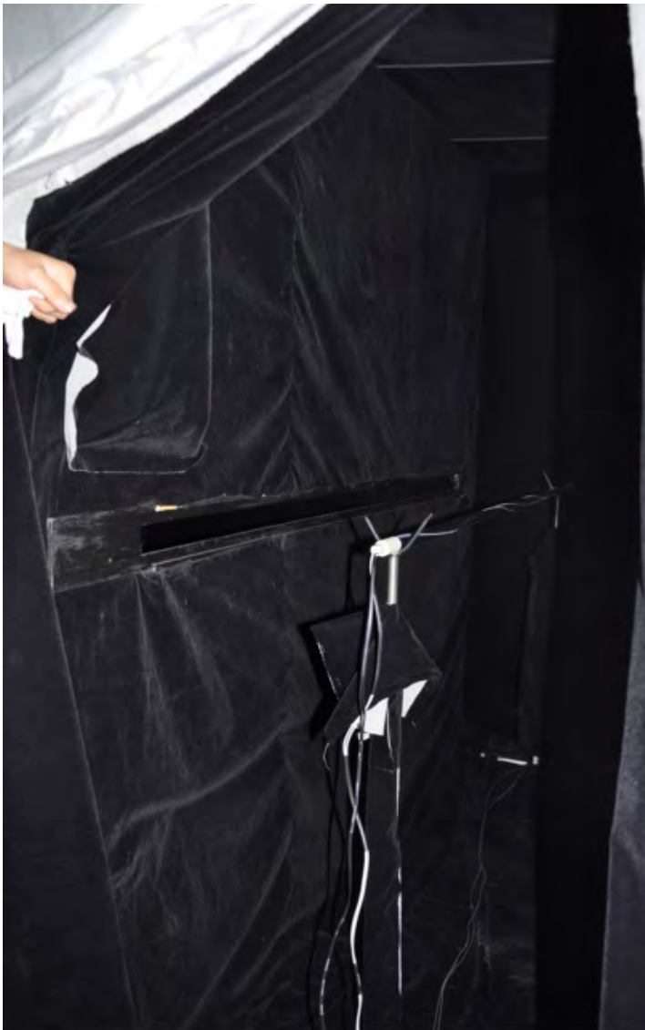
Figure C4. Lamp chamber of the lamp testing setup
