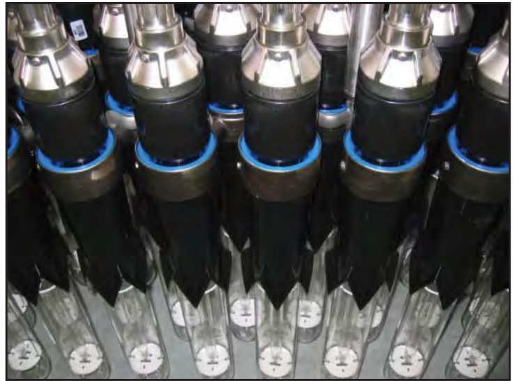
Figure 2. Vortex mixers mounted on quartz sleeves housing medium pressure UV lamps provide additional mixing and direct the low UVT water toward the high intensity light source.
